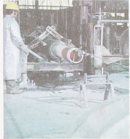
Pulling a horizontal centrifugal casting from a die.
